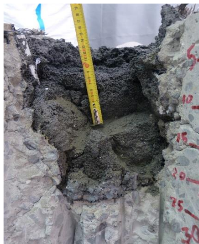
MCCI Test Results in Fukushima simulated conditions
