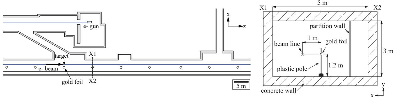
Figure 2. Experimental setup for the thermal neutron measurements at the KEK-linac.
