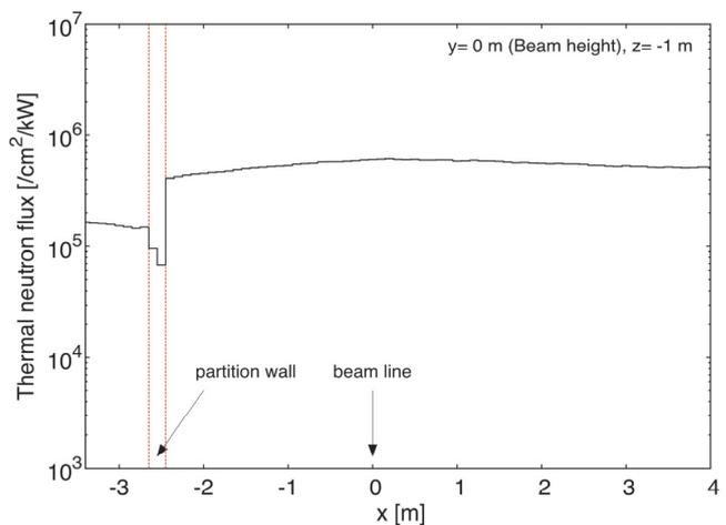
Figure 6. Calculated horizontal distribution of thermal neutrons.
