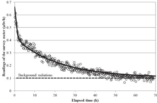
Figure 2. Readings of the survey meter at various times after irradiation on the water-filled slab phantom surface. The solid line is double exponential curve, the time parameters of which are derived from the half-life of  $^{38}\text{Cl}$  and  $^{24}\text{Na}$ .
