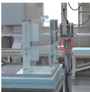
Figure 1. Photograph of the experimental setup (before covering the phantom with the cadmium container). The phantom was comprised of polymethyl-methacrylate (PMMA) walls (front wall 2.5 mm thick, other walls 10 mm thick). A circle in the photograph is the position of the neutron source.
