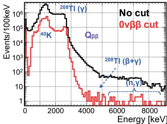
Figure 3. The observed energy spectrum in the year-2013 data. The black line shows the spectrum without analysis cuts, and the red line shows the one with all analysis cuts ( $0\nu\beta\beta$  cut). We can see some events above  $Q_{\beta\beta}$  (4.3 MeV). These events were identified as  $(n, \gamma)$  background.
