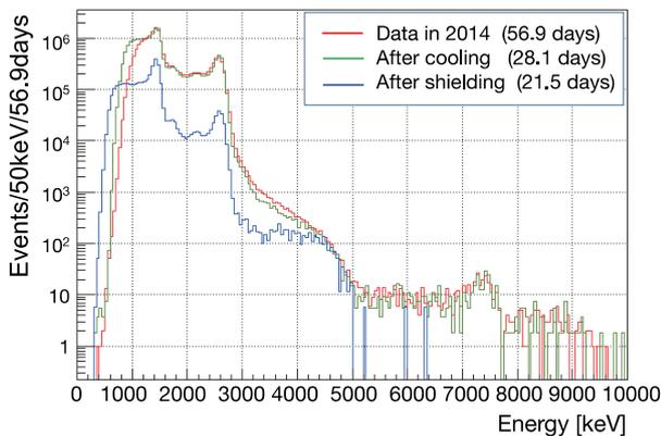
Figure 6. The observed energy spectrum without LS cut and  $^{208}\text{Tl}$  cut before and after the  $(n,\gamma)$  shield setup. The red and green histograms show the spectra before setup, and the blue histogram shows the spectrum after setup. All spectra were normalized to the event rate in 56.9 days.
