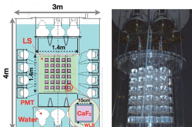
Figure 1. A schematic view of the detector. Left: A drawing of the detector from the side view. The whole detector is installed in a cylindrical stainless steel tank. Right: A photo of 96 CaF<sub>2</sub> crystals which are immersed in LS.
