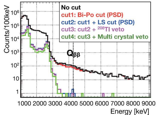
Figure 7. The energy spectrum after  $(n,\gamma)$  shield setup in the 21.5 days live-time measurement by applying various analysis cuts, i.e. the Bi-Po cut, the LS cut, the  $^{208}\text{Tl}$  veto, and the multi crystal veto that are described in section 3.2, 2, 3.3, 3.3, respectively. The green histogram shows the spectrum obtained with all analysis cuts. There are no events in the region of interest ( $Q_{\beta\beta-1\sigma}^{+2\sigma}$ ; 4170-4480 keV).
