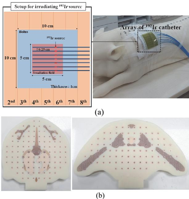
Figure 2. Experimental setup for measuring the dose distribution: (a) <sup>192</sup>Ir catheter setup for irradiating at the 5<sup>th</sup> slice, (b) RPLGDs inserted in the 5<sup>th</sup> and 25<sup>th</sup> slices of the minipig physical phantom.
