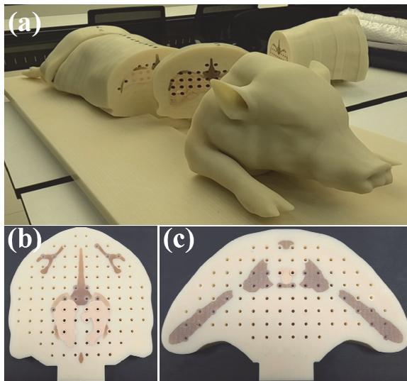
Figure 1. Geometry of the minipig physical phantom: (a) the minipig physical phantom sliced into 27 slices, cross section of the (b) 5<sup>th</sup> and (c) 25<sup>th</sup> slices.
