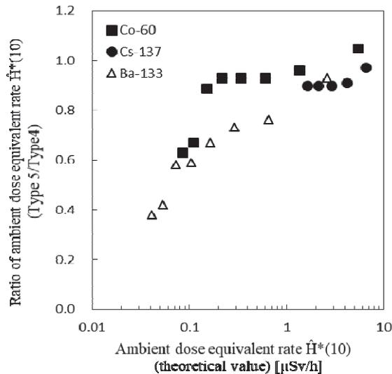
Figure 6. Ratio of ambient dose equivalent rate between the type 4 and 5 pocket geigers.
