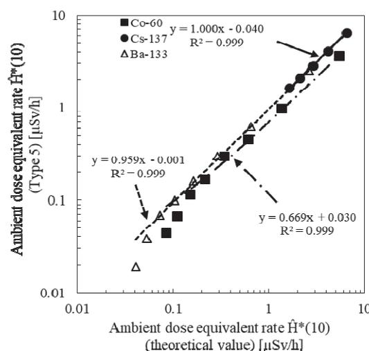
Figure 5. Ambient dose equivalent rate. Characteristics of the type 5 pocket geiger.
