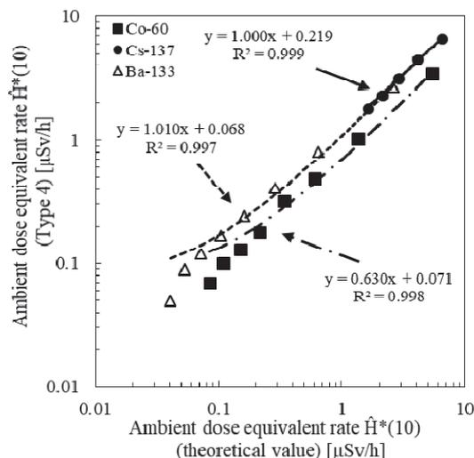
Figure 4. Ambient dose equivalent rate. Characteristics of the type 4 pocket geiger.
