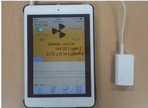
Figure 1. Photograph of a wired type 4 pocket geiger.
