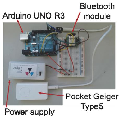
Figure 2. Photograph of a type 5 pocket geiger and a wireless transmitter system.
