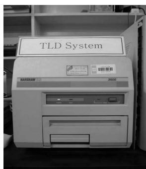
Fig. 3 GR-200 TLD rods and Harshaw model 3500 TLD reader used in the measurement
