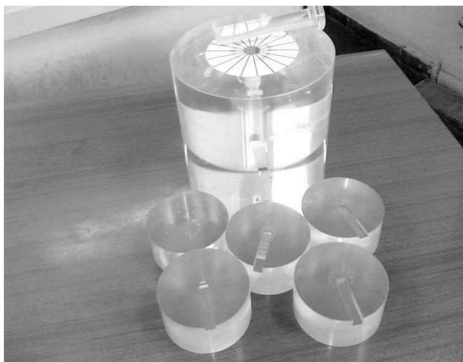
**Fig. 4** The phantoms used for dosimetry in the present work, 10cm diameter by 10cm high and 20cm diameter by 20 cm high PMMA cylinders
