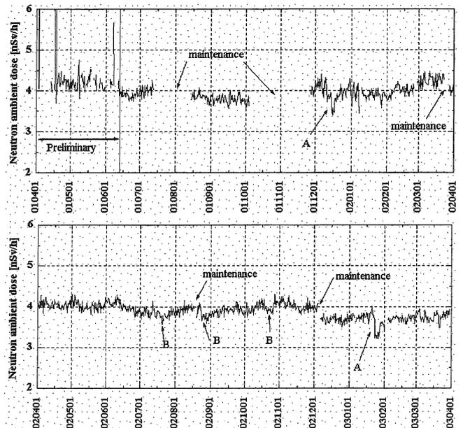
Fig.7 Neutron ambient dose equivalent measured by the rem counter from April 2001 to March 2003.
