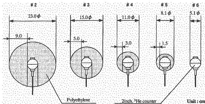
Fig. 2 Cross-sectional view of <sup>3</sup>He-loaded multi-moderator detectors
