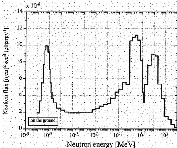
Fig. 6 Initial guess spectrum for the SAND-II code used in this study obtained by Goldhagen et al. [7].
