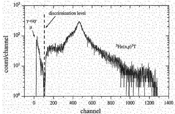
Fig. 4 Pulse-height discrimination of rem-counter and Bonner ball
