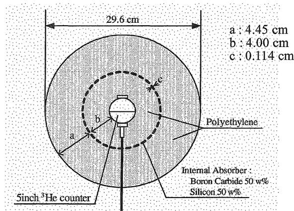
Fig. 1 Cross-sectional view of the rem counter
