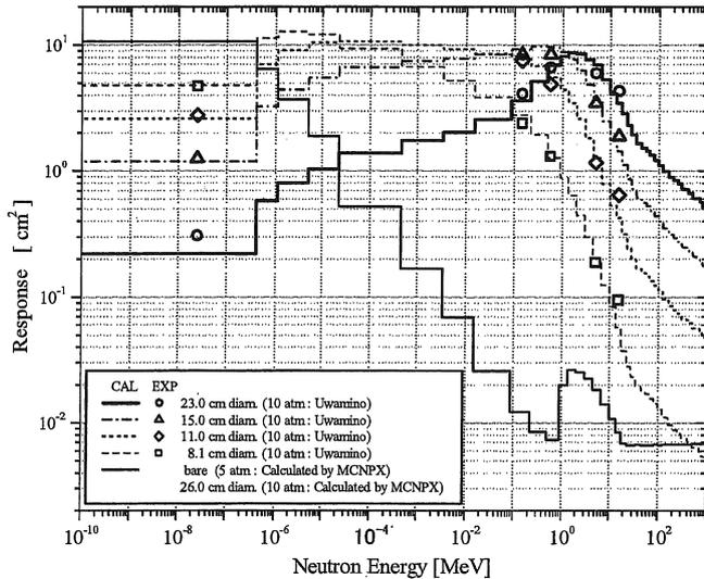
Fig. 5 Response functions of  $^3\text{He}$ -loaded multi-moderator detectors calculated with the ANISN code [5] by Uwamino et al. [3] and the MCNPX code [6]
