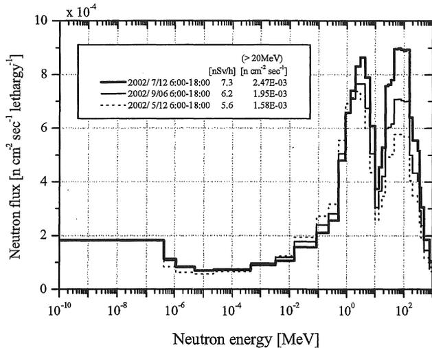
Fig. 8 Comparison of neutron energy spectra on three different days obtained by the Bonner ball with the SAND-II unfolding.
