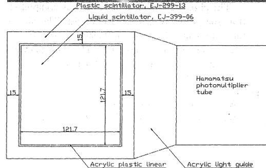
Fig. 3 Picture (upper) and configuration (lower) of the phoswich neutron detector
