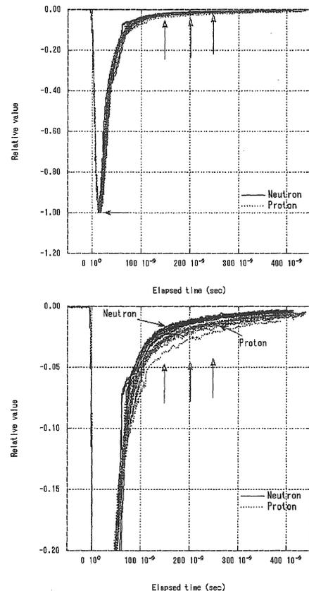
**Fig. 4** Neutron and proton pulse shapes normalized at peak value (top), and magnified signal tails from 0 to -0.2 V (bottom)
