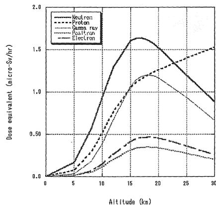
Fig. 1 Particle dose equivalent at high altitude calculated with LUIN2000<sup>1)</sup>
