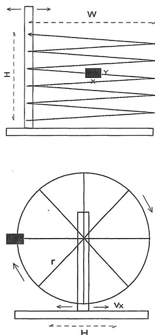
Fig. 1 XZ-linear (above) and rotational-linear (below) scanning methods. The filled area XY represents the photon beam.
