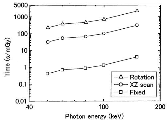
Fig. 3 Typical required time for 1-mGy irradiation at the fixed, XZ-linear and rotational-linear scanning methods at BL38B1 beamline
