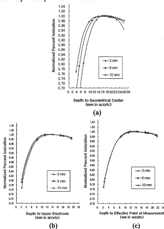
**Fig. 6** Shift of the EPM in each chamber under the condition of 6 MV photon beam.
