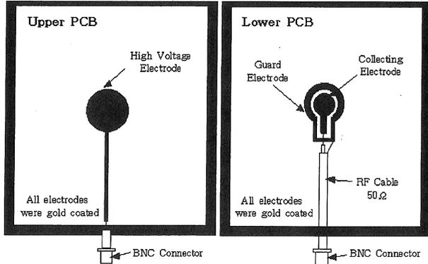
Fig. 1 Schematic diagrams of the printed circuit boards.
