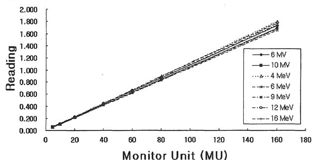
**Fig. 5** Linearity of the ionization chamber with a volume of 0.9 cc.
