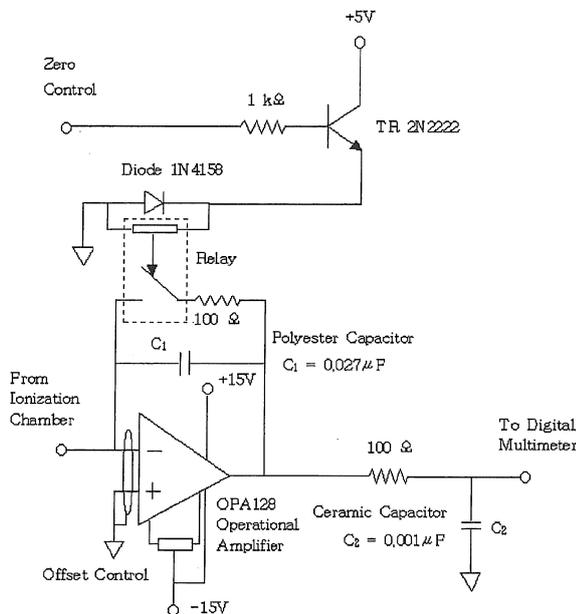
Fig. 3 Schematic diagram of charge to voltage converter.
