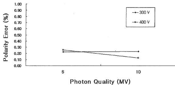
Fig. 8 Polarity effect for photon beams in the ionization chamber with a volume of 0.9 cc.
