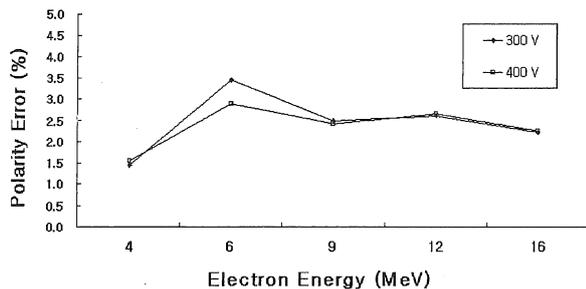
Fig. 9 Polarity effect for electron beams in the ionization chamber with a volume of 0.9 cc.
