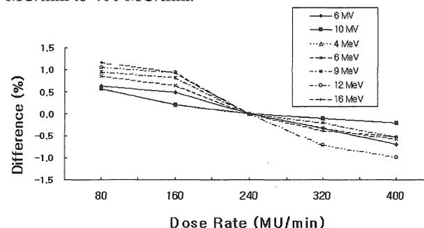
**Fig. 7** Dose rate effect of the ionization chamber with a volume of 0.9 cc.
