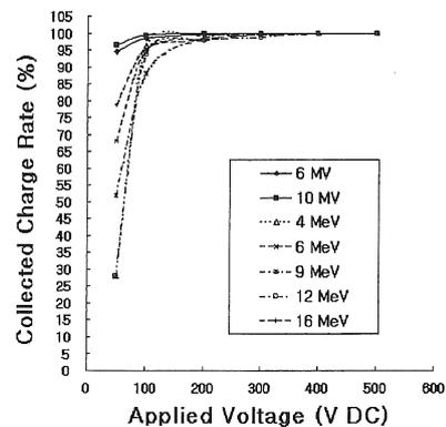
Fig. 4 Saturation voltage of the ionization chamber with a volume of 0.9 cc.
