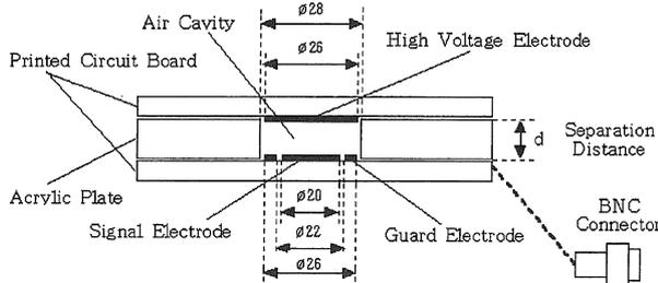
Fig. 2 Cut-away view of the parallel plate type ionization chamber. Separation distance  $d$  : 3 mm, 6 mm, 10 mm
