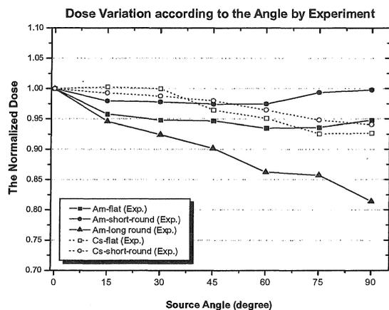
Fig. 10 The current variations measured by experiment with the incident source angle
