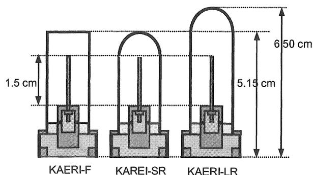
Fig. 1 The cross-sectional view of the ionization chamber with various window type designed and simulated.
