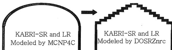
Fig. 3 The approximation used for reproducing the round-type window in DOSRZnrc
