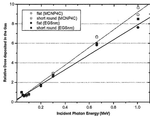
Fig. 4 The current variations of the ionization chamber by changing incident gamma-ray energy from 40keV to 1MeV calculated by EGSnrc, MCNP4C
