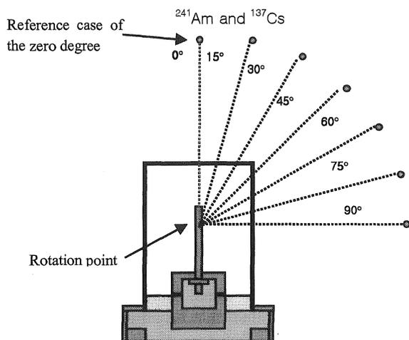
Fig. 5 The variation of the source angle incident on the ionization chamber
