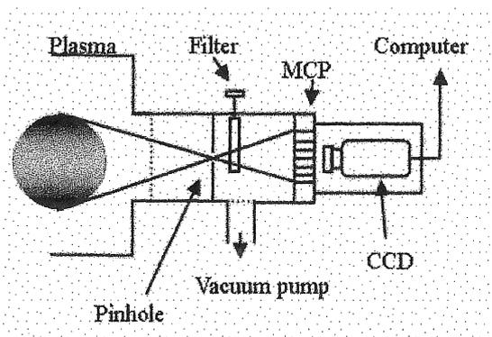
Fig. 1 The apparatus of soft x-ray imager
