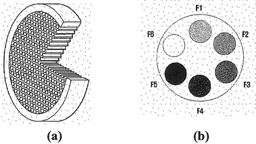
**Fig. 2** (a) Microstructure of the MCP (b) the changeable filter array; F1~F6 are the main aluminum filters of different thicknesses, and F5 and F6 are the shielded and the open holes.
