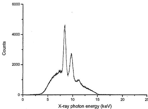
**Fig. 4** The x-ray spectrum of the x-ray generator (15 kV, 0.3 mA) measured by a Si pin-diode with a 2048-ch MCA. See the three L-edges of the tungsten, which are  $L_{\alpha} = 8.37$  keV,  $L_{\beta} = 9.82$  keV, and  $L_{\gamma} = 11.29$  keV in sequence.
