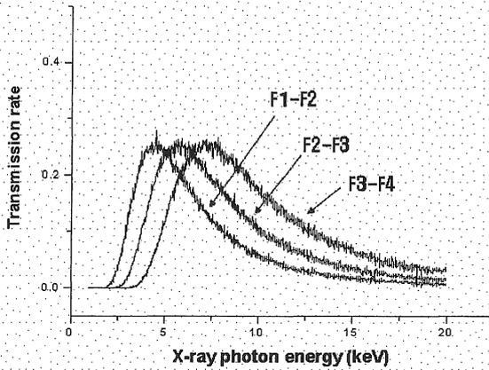
**Fig. 3** Transmission rates of x-ray photons with a constant spectrum after filtration and subtraction. Three curves are obtained by using three pairs of filters, F1-F2, F2-F3 and F3-F4, and they have a peak at 4.38, 5.61 and 7.18 keV.
