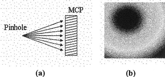
**Fig. 5 (a)** the schematic geometry of the x-ray beam and the MCP channels with a bias angle, **(b)** the calculated results of pixel brightness due to an isotropic point source located at the pin hole position of the imager
