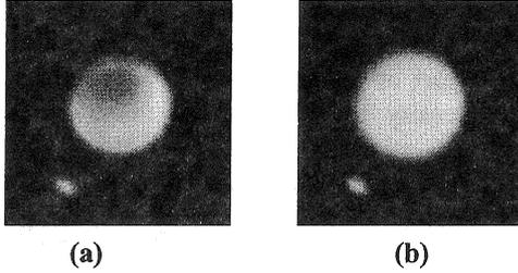
Fig. 6 (a) the measured and (b) LUT-corrected image of an x-ray generator located at the same position as the pin hole
