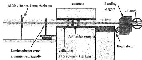
Fig. 6 The arrangement of fast neutron profiling
