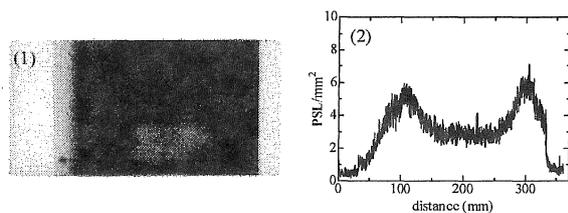
Fig. 7 (1) The fast neutron image measured by the IP-aluminum method with activation samples and semiconductor samples in, (2) The horizontal PSL distribution along the vertical center
