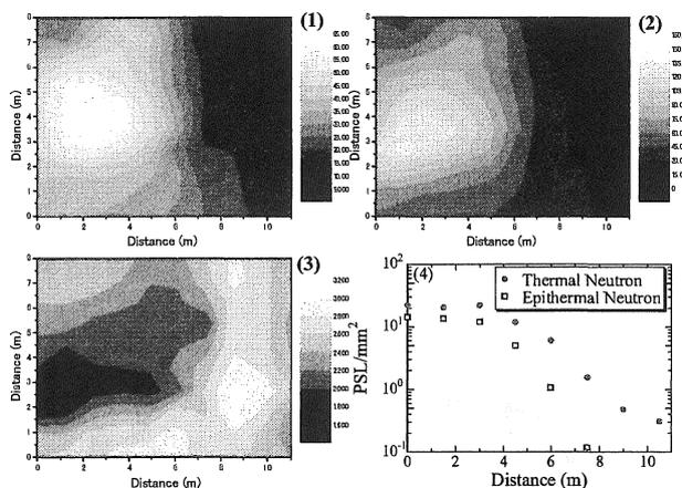
Fig. 5 (1) Thermal neutron spatial distribution, (2) Epithermal neutron spatial distribution, (3) Cd-ratio spatial distribution, (4) Thermal and epithermal neutron distributions at center of downstairs
