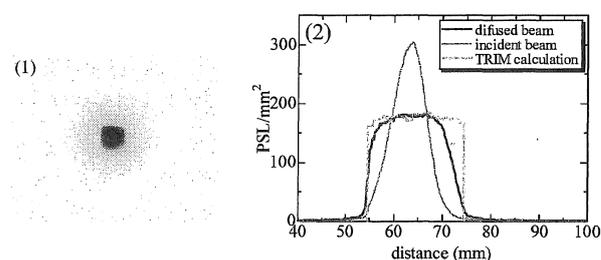
Fig. 9 (1) The proton image measured by IP and copper foil on a semiconductor chip, (2) The vertical PSL distribution along the horizontal center
