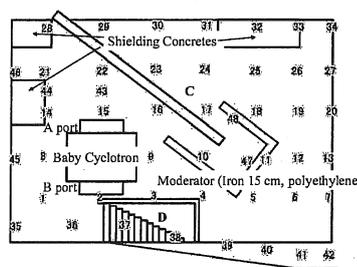
Fig. 3 Arrangement of activation foils in TR.1 48 pairs of gold foils (bare and Cd-covered)
