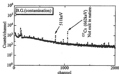
Fig. 1  $\gamma$ -ray spectrum of lead blocks contaminated with a weak activity of  $^{137}\text{Cs}$
