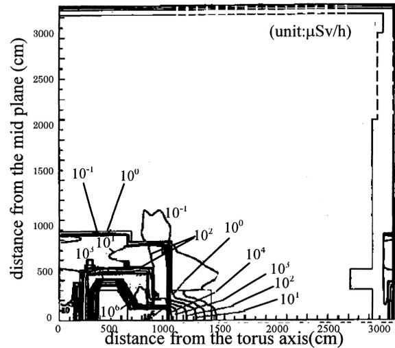
**Fig.7** Dose rate distribution at one month after shutdown of 8000sec DT operation with neutron production rate  $10^{20}$  n/s in JT-60SU.
