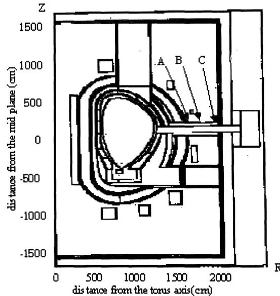
**Fig.9** Evaluation points (A,B,C) for the ratio of the high energy neutron fluxes in 2-D torus model of ITER.<sup>(5)</sup>
