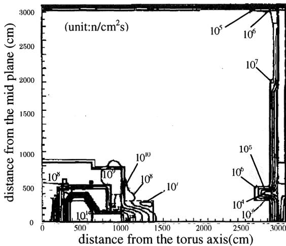
**Fig.3** Total neutron flux distribution during DT operation of neutron production rate  $10^{20} \text{ n/s}$  in JT-60SU
