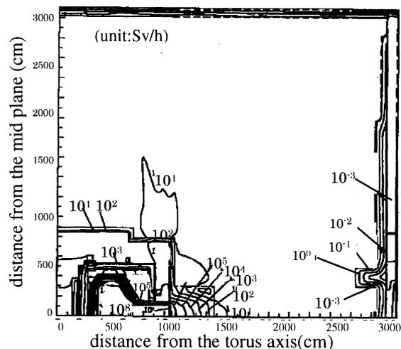
**Fig.5** Dose rate distribution during DT operation of neutron production rate  $10^{20} \text{ n/s}$  in JT-60SU
