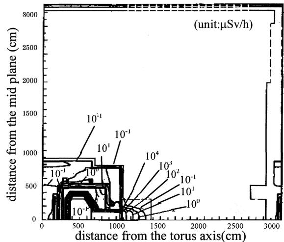
**Fig.8** Dose rate distribution at one year after shutdown of 8000sec DT operation with neutron production rate  $10^{20}$  n/s in JT-60SU.
