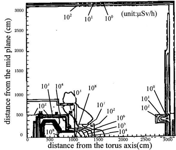
**Fig.6** Dose rate distribution at one day after shutdown of 8000sec DT operation with neutron production rate  $10^{20}$  n/s in JT60SU.
