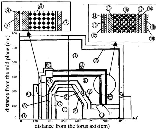
**Fig. 2** Expanded two dimensional RZ torus model from the torus center to the cryostat in JT-60SU
